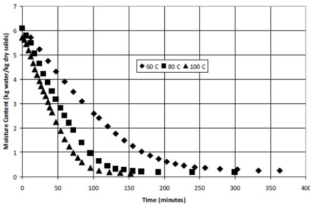
**Figure 3.** Representative drying curves of gold kiwifruit slices with an air velocity of 0.20 m/s at ambient humidity and different temperatures.
