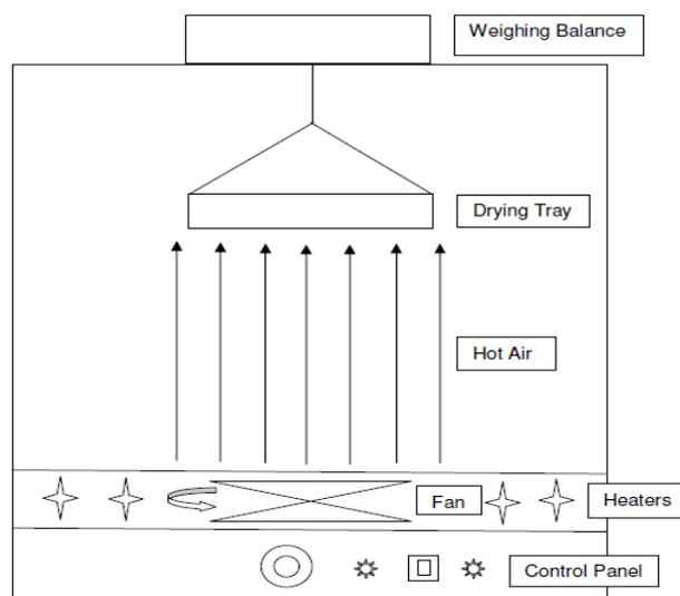
**Figure 1.** Schematic diagram of the hot air dryer used in the experiments.
