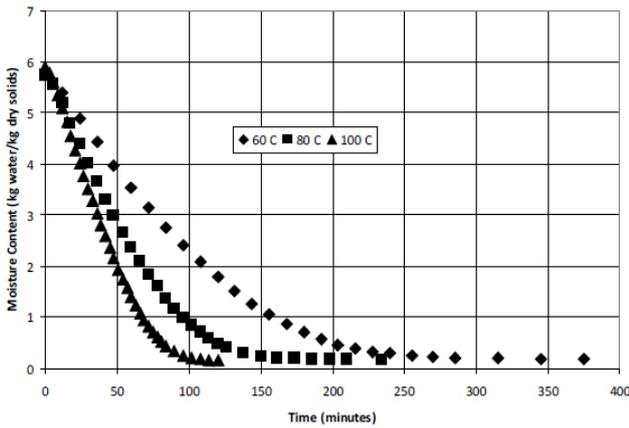
**Figure 2.** Representative drying curves of green kiwifruit slices with an air velocity of 0.20 m/s at ambient humidity and different temperatures.
