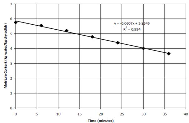
**Figure 6.** Drying curve of green kiwifruit slices with an air velocity of 0.20 m/s at ambient humidity and temperature of 80°C for replication 2 of green kiwifruit (Data 4) showing the CRP drying rate regression.
