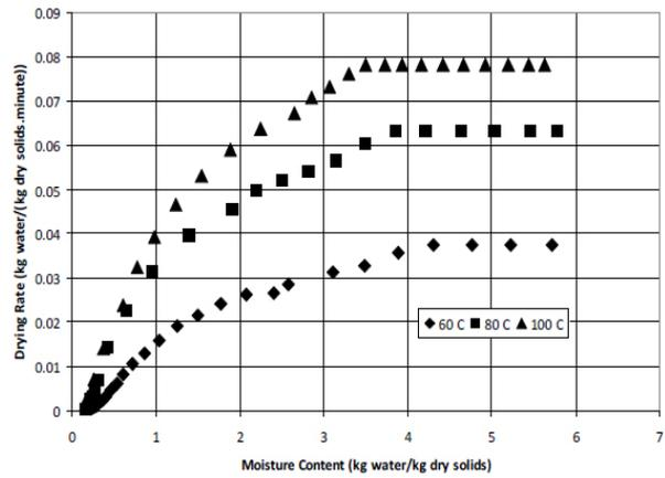
**Figure 5.** Representative drying rate curves of gold kiwifruit slices with an air velocity of 0.20 m/s at ambient humidity and different temperatures.
