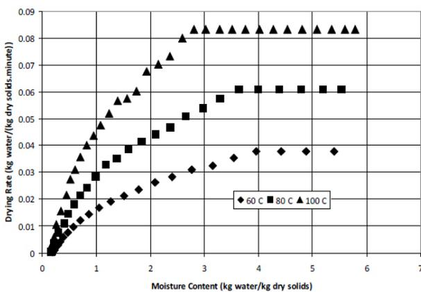
**Figure 4.** Representative drying rate curves of green kiwifruit slices with an air velocity of 0.20 m/s at ambient humidity and different temperatures.
